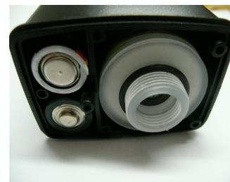
Two AA 1.5 volt Alkaline Batteries Type MN1500, LRG 1.5 or similar must be installed in the TEK-OX to the correct way to enable it to operate.
