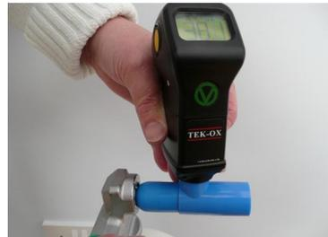
**Mate the Quick-Ox to the cylinder outlet**
